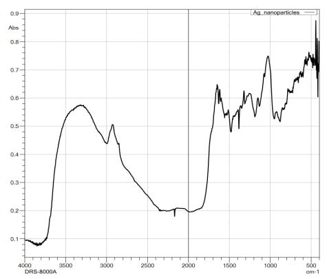
Figure 7. FT-IR Spectral Representation of Synthesized AgNPs.
