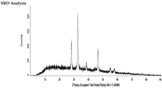
Figure 8. XRD pattern of biosynthesized silver nanoparticles.
