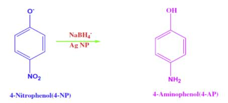
Figure 12. Schematic representation of the performance of Synthesized Silver Nanoparticles (AgNPs) as catalysts in the reduction of 4-nitrophenol to 4-aminophenol by NaBH<sub>4</sub>.
