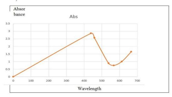
Figure 6. UV-Vis Spectra of Synthesized AgNPs.
